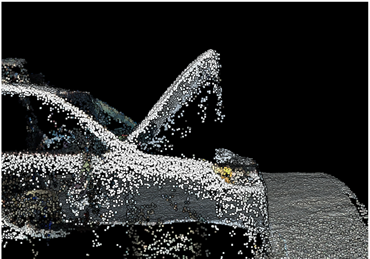
Figure 4.2.12.3: the point cloud is trying to merge the gap because the engine hood is a concave shape.
