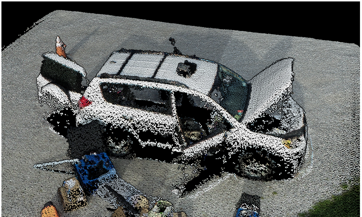
Figure 4.2.12.12: the lower half of the door has no point cloud. This might be because those surfaces are facing below the horizon.
