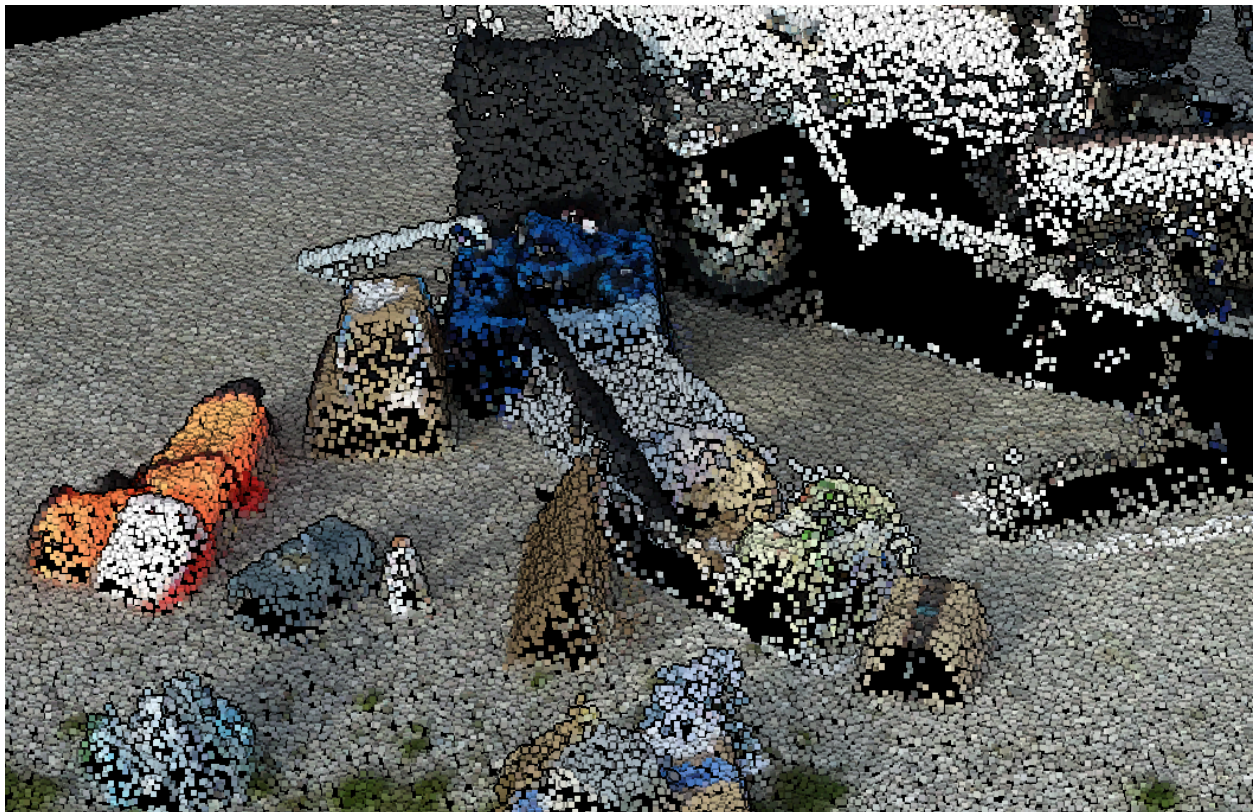
Figure 4.2.10.2: Even though the box is a concave shape, the point cloud is still able to generate the shape.
