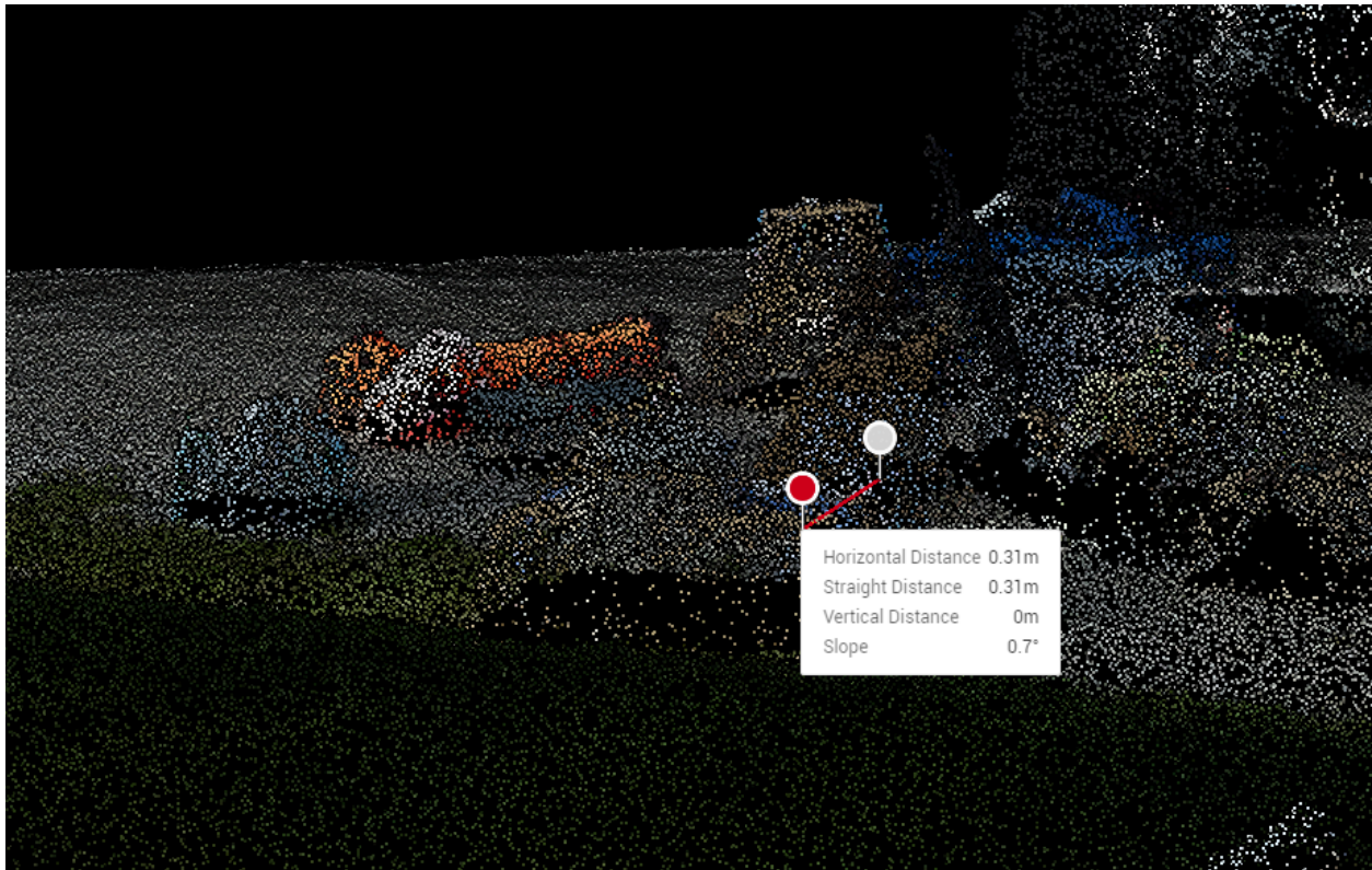
Figure 4.2.1.4: change the perspective to verify that two points are on the same height.
