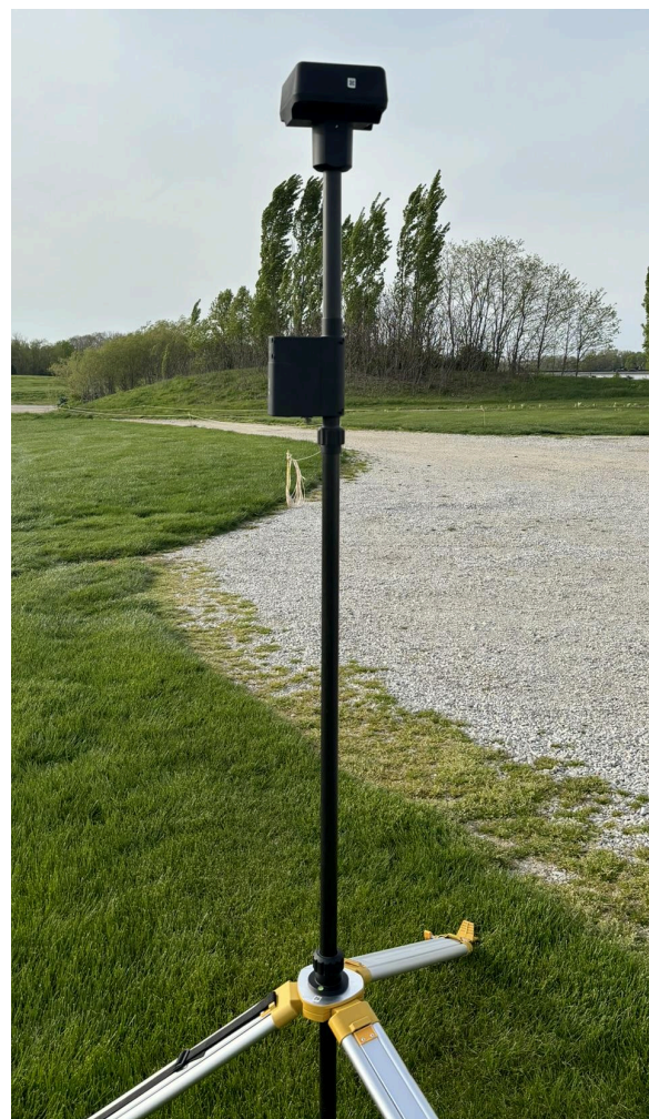
Figure 2.1.3.2: DJI D-RTK 2 set up.
