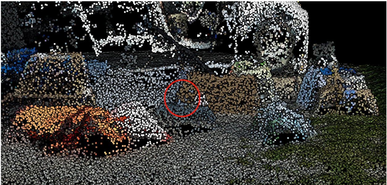
Figure 4.2.15.2: It's very hard to see the cup because there are not many points.
