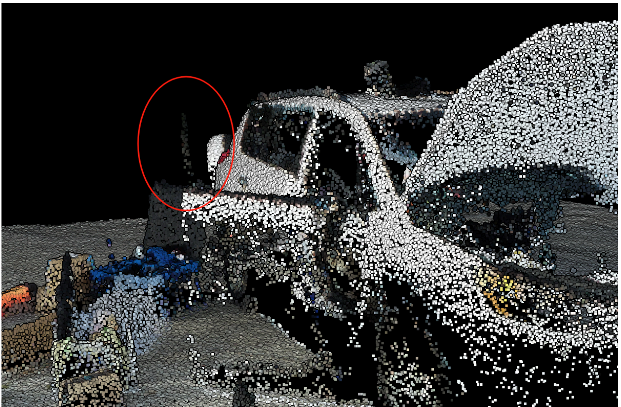
Figure 4.2.12.5: The black points are the window frame of the front door. There is no window, only the part of the frame. The top part of the frame is missing.
