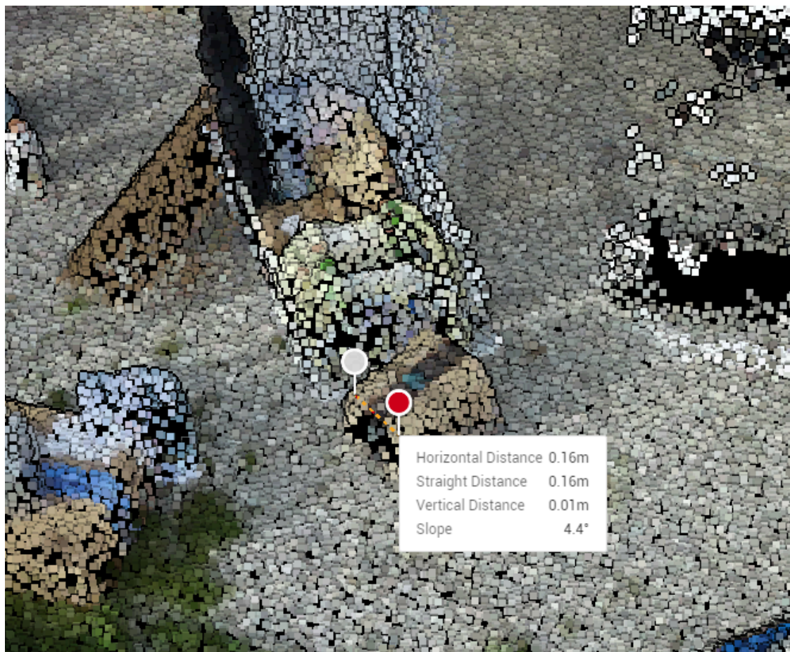
Figure 4.2.1.6: measured length is 16 cm. Actual length is 21 cm. Two sides of the box are not straight up, making its cross section into a trapezoid.
