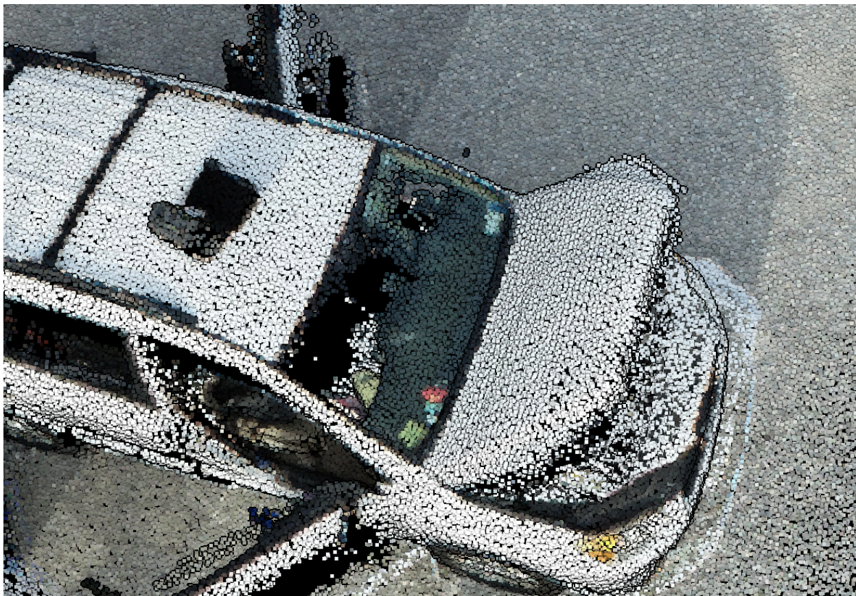
Figure 4.2.12.7: This is the top view of the front windshield, but the windshield doesn't have any points. The dark gray points are from the dashboard.
