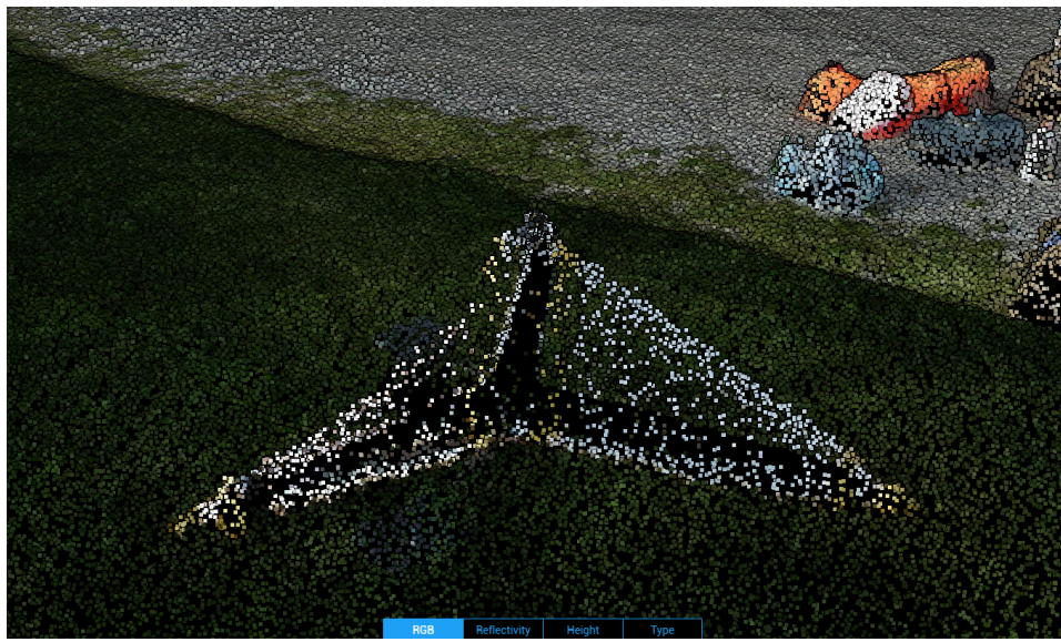
Figure 4.2.7.2: The tripod base formed a concave shape, and the point clouds are trying to merge the gap.
