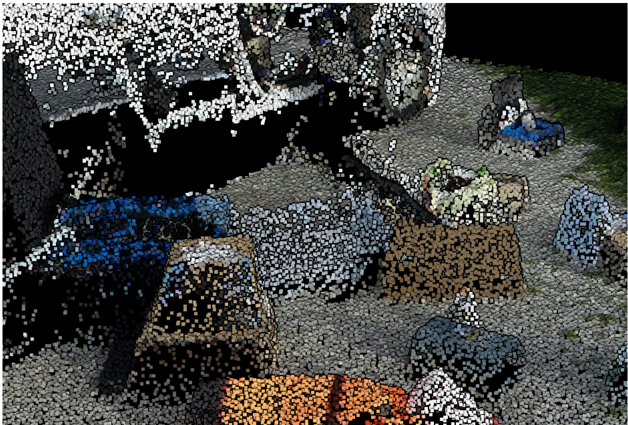
Figure 4.2.11.3: the lid is regenerated as a box. The space under the lid is covered by the wall of point cloud, and the top is opened.
