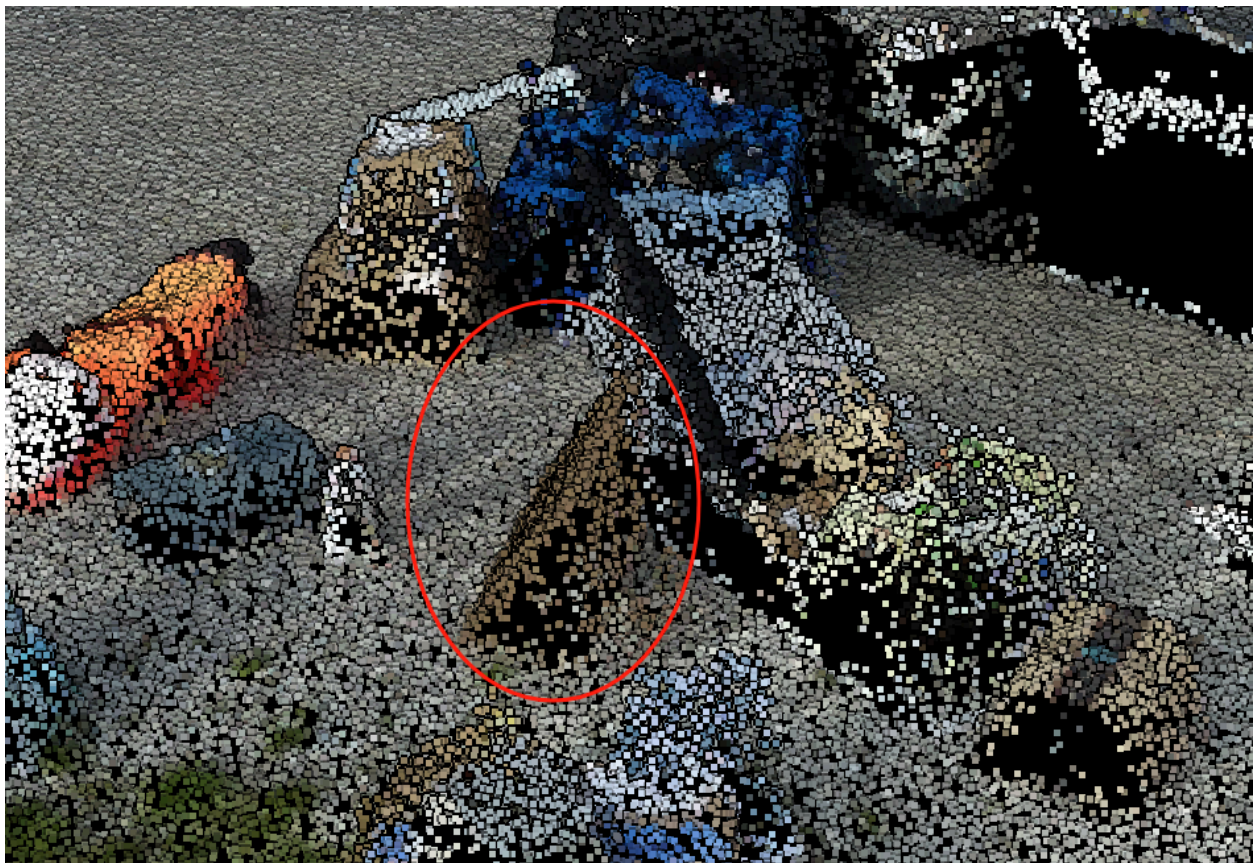
Figure 4.2.18.2: the right side of the laminate flooring board formed a concave shape and the point cloud merged it.
