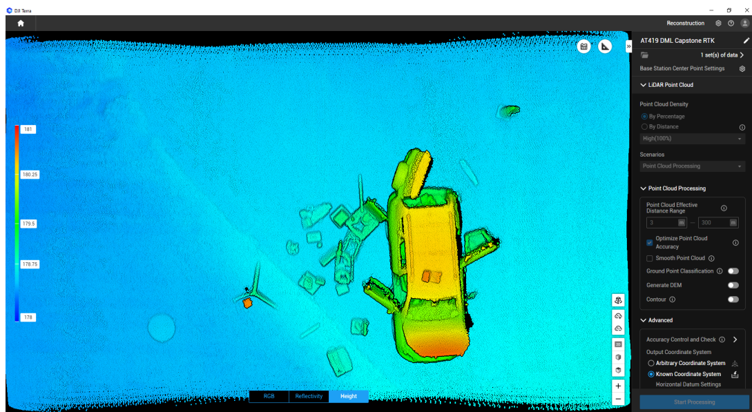
Figure 4.1.9: Point Cloud Processing, Height top view.
