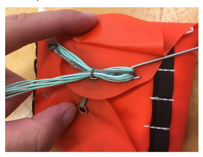
Ise the hook to pull the suspensions lines through the rest of the elastic holes. Make sure they don't overl
