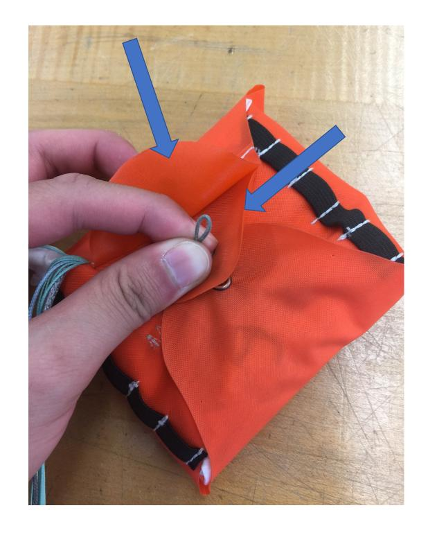
24. Use a hook to pull a little section of the suspension lines through the elastic loop, like shown in the picture.
