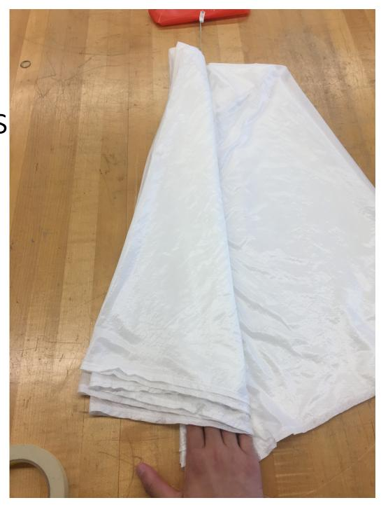
15.1. Repeat step 14, until the half part of the parachute are folded in the 10 cm wide section
