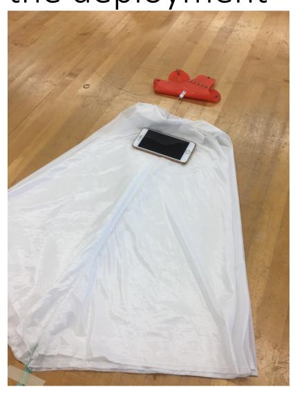
O. Remove the anchor. Fold the top of the parachute in the zigzag format (1 ke what's shown in the picture. Finally, it should have 4 gores on each side 2)(3)
