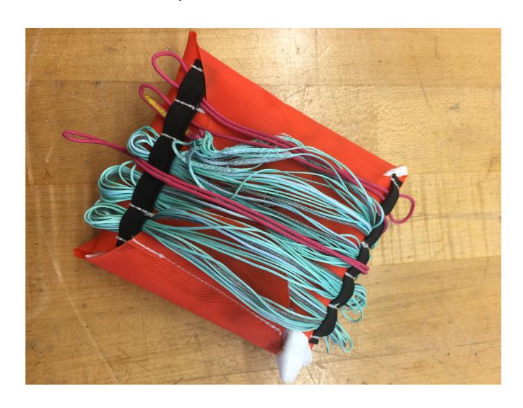
. Put the parachute and the hook into the pouch. Write the name, date, d time on the tape FIRST, then stick the tape to the bag.
