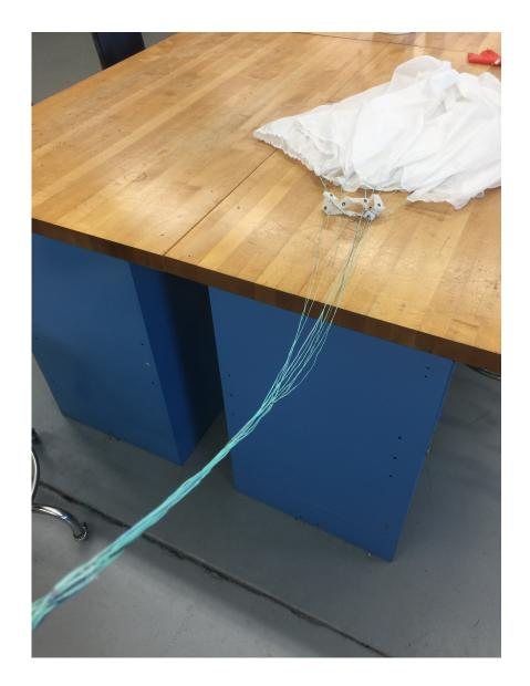
I the spot where the suspension line and the canopy connect, then find the two spots that are neighbors ( In two spots together (2), then find the folding edge of the canopy (3). Now the two spots is at the central In e folding edge is like the edge of the page of a book.
