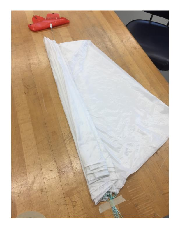
15.3 Flat the parachute by pushing it all the way down.
