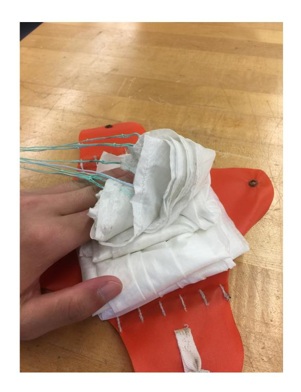
22. Put the break into the deployment bag (1). Make sure the suspension lines that are outside of the bag have the equal length. Put the extra suspension line into the bag.
