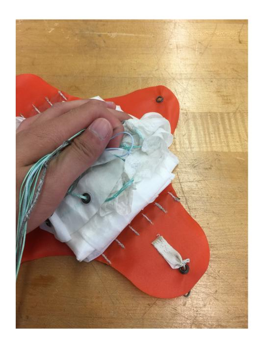
23.1 Make the elastic loop go through the holes on the deployment bag.
